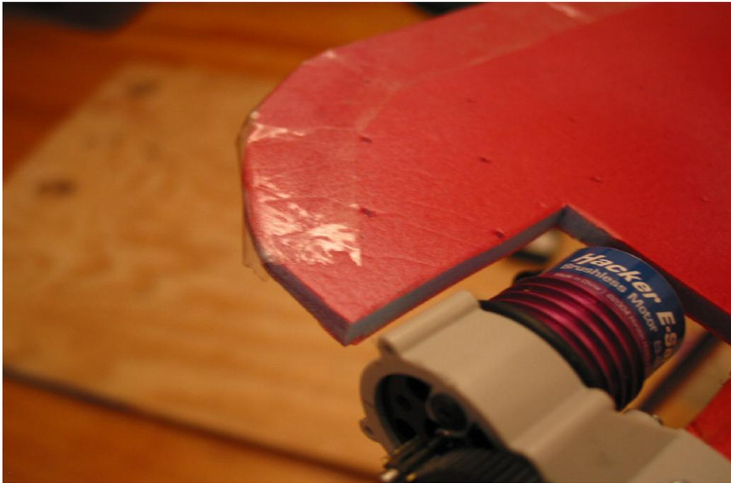
Run clear packing tape down the bottom of the fuselage to behind the wing. Run another piece just behind the motor, top to bottom. This will add lots of strength for landings and crashes, with very little weight gain.
