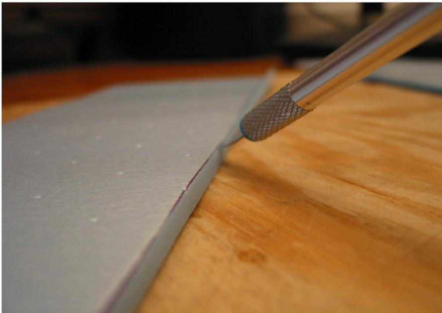
For ailerons, cut a 45 degree angle along the inside edge. Do the same on the wing where they will hinge.
