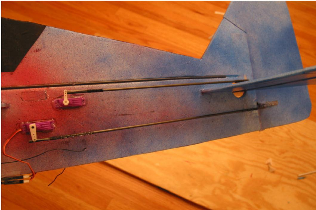
Carbon fiber and music wire again. If you don't have CF, use wire that is braced through straws glued to side about 1 inch long each.
