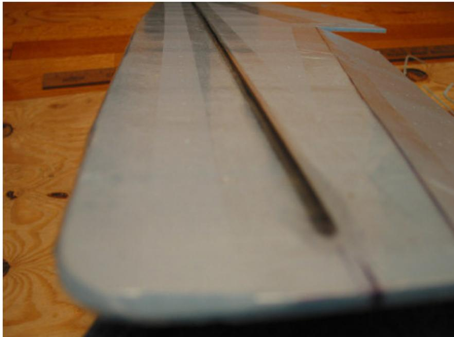
Run another piece of clear packing tape down the leading edge of the wing. This will protect it and help keep its shape.
