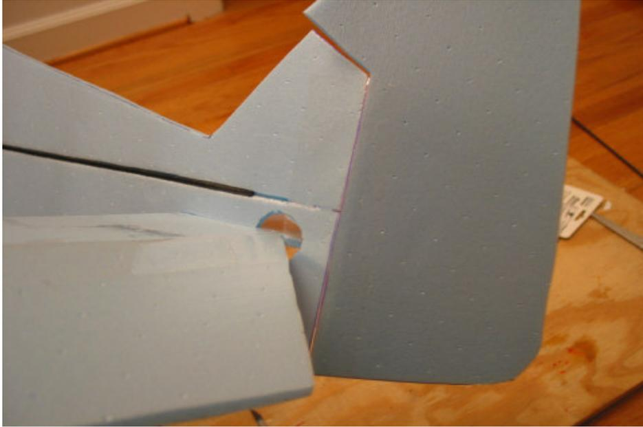
Add tape to rudder and attach.
