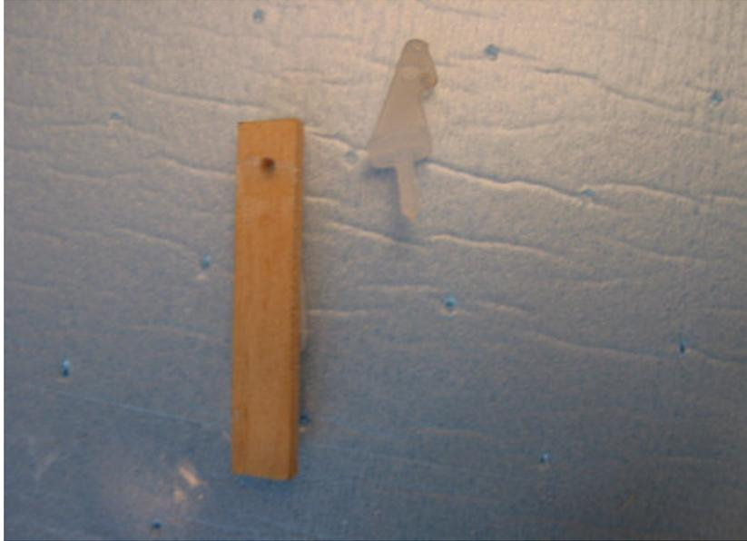
I use the dubro control horns and a small piece of basswood about 1/8in x 2-3 inches long. Drill a small hole for the control horn.
