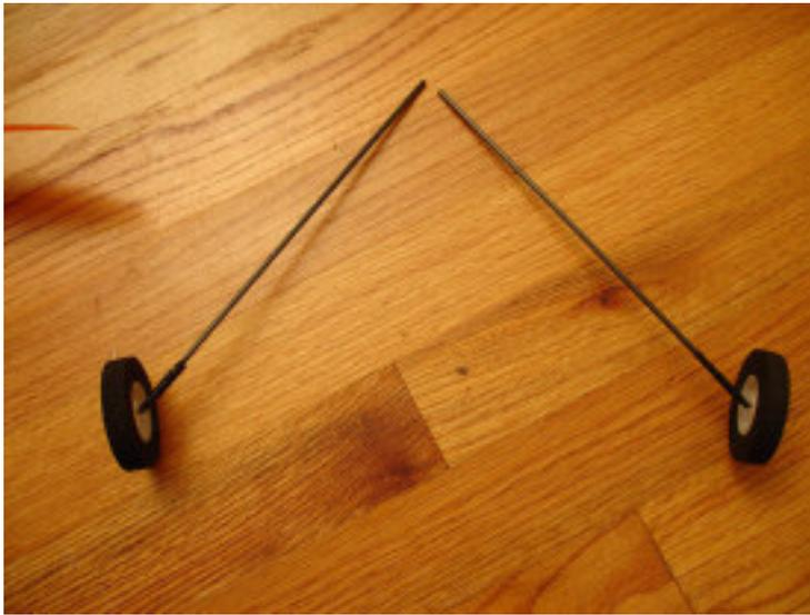
To add landing gear, cut two pieces of aprox.  $\frac{3}{16}$  in (2.5mm) solid carbon fiber rods 8-8  $\frac{3}{4}$  in long (20-21.5cm) Cut two pieces of music wire 1  $\frac{1}{2}$  in. (4 cm) long, bend them to the desired angle, wrap with thread and CA glue. Add 2 inch (5cm) wheels.
