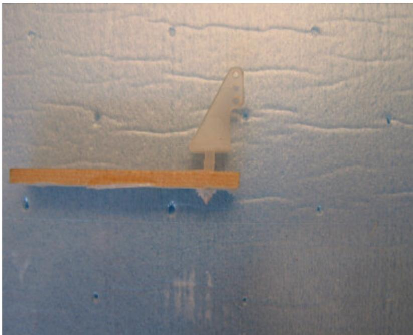
Push horn through hole and glue. (Shown partially inserted)
