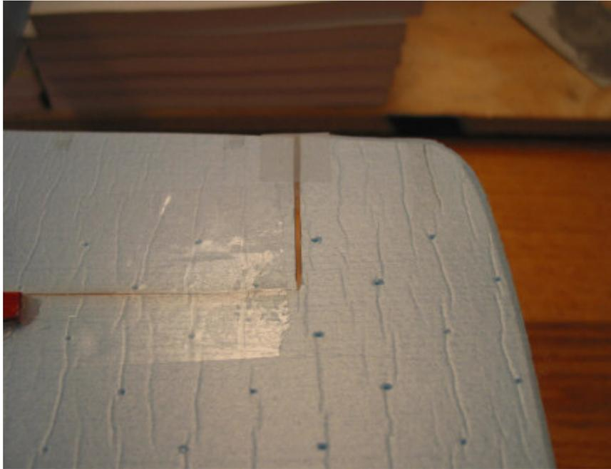
Before gluing wood brace to elevator, straighten them by putting removable tape on the leading edge. After epoxy dries, remove tape and they will be even.
