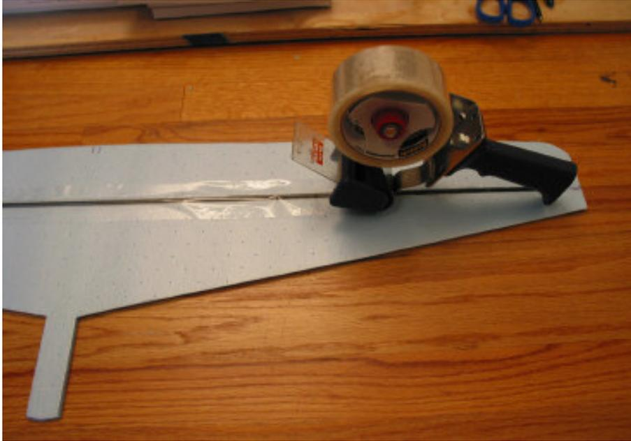
Using clear packing tape, place a strip down along the spar on both sides of the wing.
