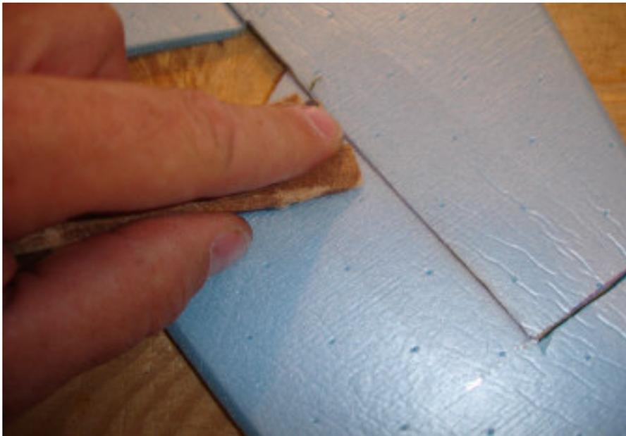
Using medium grade sandpaper, lightly roughen up the packing tape on the elevator. It'll give the wood stick good adhesion when glued.
