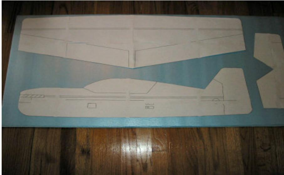
Tape tiled plans together to make full size plan. With full size or tiled plans that have been taped, cut out the “Nasty” and tape to the foam. Trace along the outside edge and remove plans. Using a sharp new #11 exacto knife, cut out the “Nasty” holding the knife straight. Take your time and make smooth long cuts.
