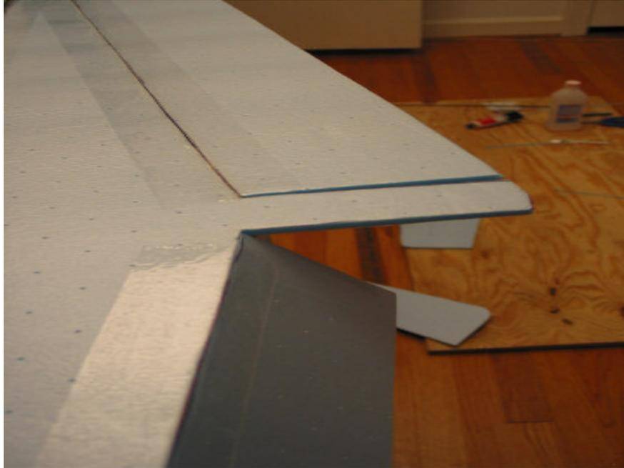
Place clear packing tape along the aileron with it at a 45-50 degree angle.
