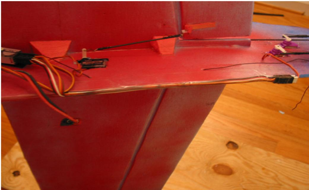
Add servo extensions of 12 inch each if needed, from rear servos to receiver.
