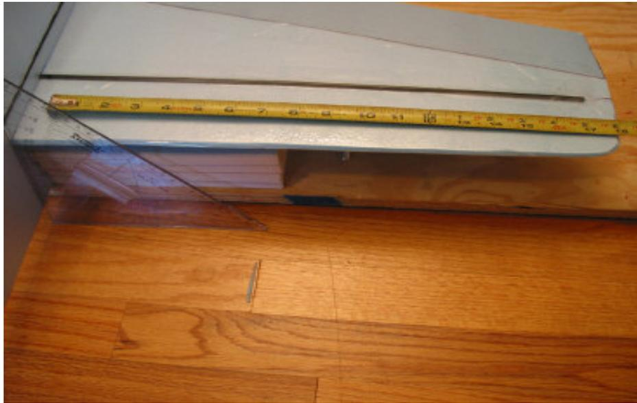
Prepare wing for gluing by leveling the wing with books and using a right angle to check wing is straight and level.
