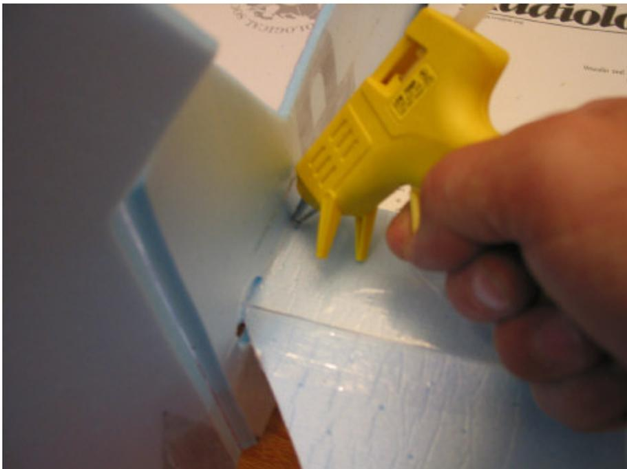
Glue stab into place with hot glue or 5 minute epoxy. Add tape to elevators and attach at 45-50 degree angle.
